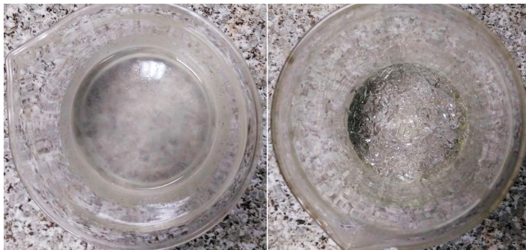
Figure 6. Macro-observations of SAP particles saturated with a solution of mixing and a superplasticizer admixture ( left ) and saturated with mixing water with no admixture ( right ) show the synergistic effect between SAP and superplasticizer.
