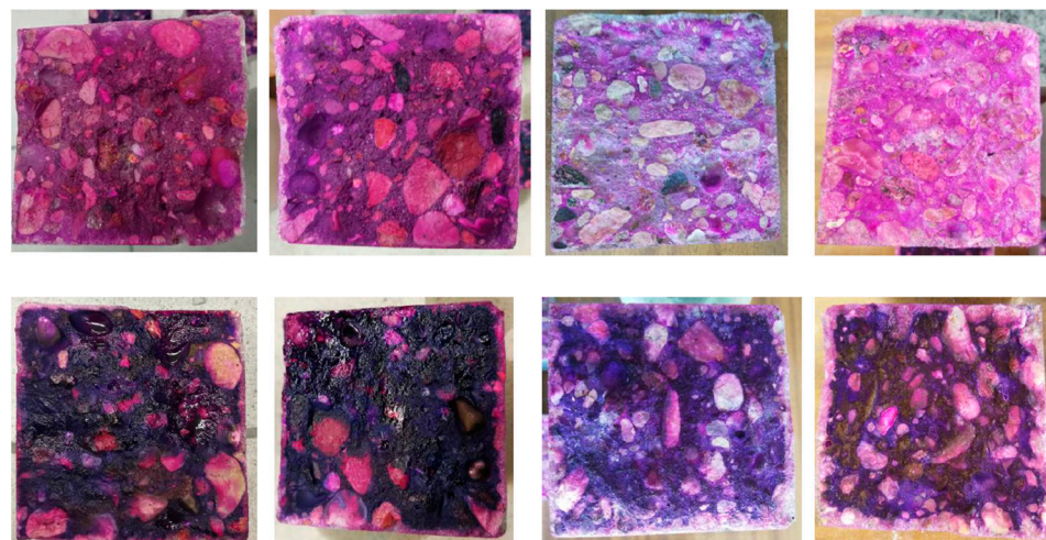
Figure 7. Depth of carbonation determined with the indicator recommended in the EN 13295:2004 standard [35], i.e., phenolphthalein (top row), and with an extra indicator, i.e., thymolphthalein (bottom row) of concrete SAP-50 after 14, 28, 56 and 70 days (from left) in 1% of CO 2 .
