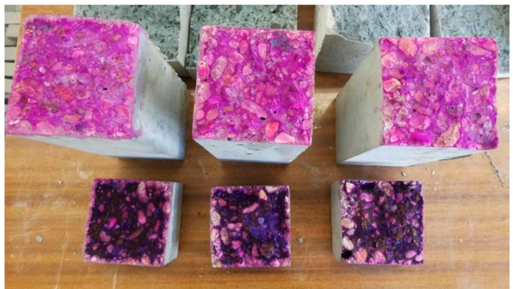
Figure 4. Concrete specimens are used to test the depth of carbonation with the indicator recommended in the EN 13295:2004 standard [35], i.e., phenolphthalein (indicating pH ~8.5)—upper row
