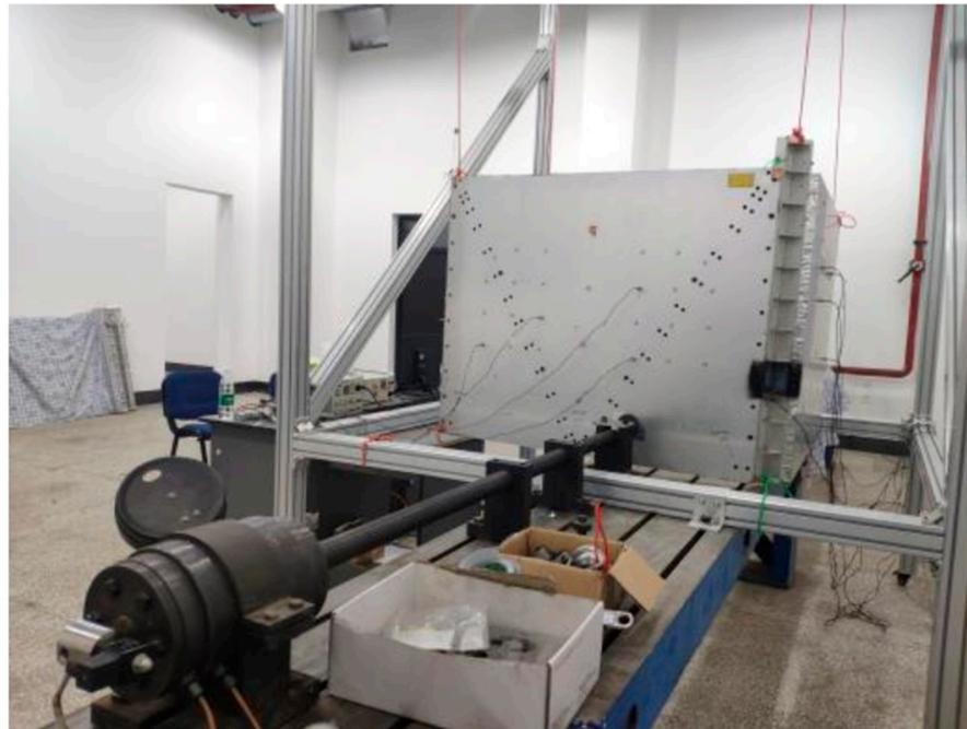
**Figure 2.** Shock test state of coupling plate structure.
